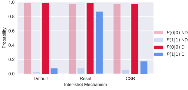
Figure 14: Measurement probabilities of the attacker when the victim circuit’s individual qubits are driven from |1\rangle to |3\rangle (D) and when they are not driven (ND) following the measurement of the victim circuits. The figure shows the attackers’ measurement probabilities for different inter-shot mechanisms. P(x|y) is the probability of x as the measurement result for the attack circuit under the condition that the measurement result of the victim circuit is y and then followed by the inter-shot mechanism.
