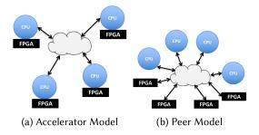
Fig. 1. Example FPGA placement in datacenters.
